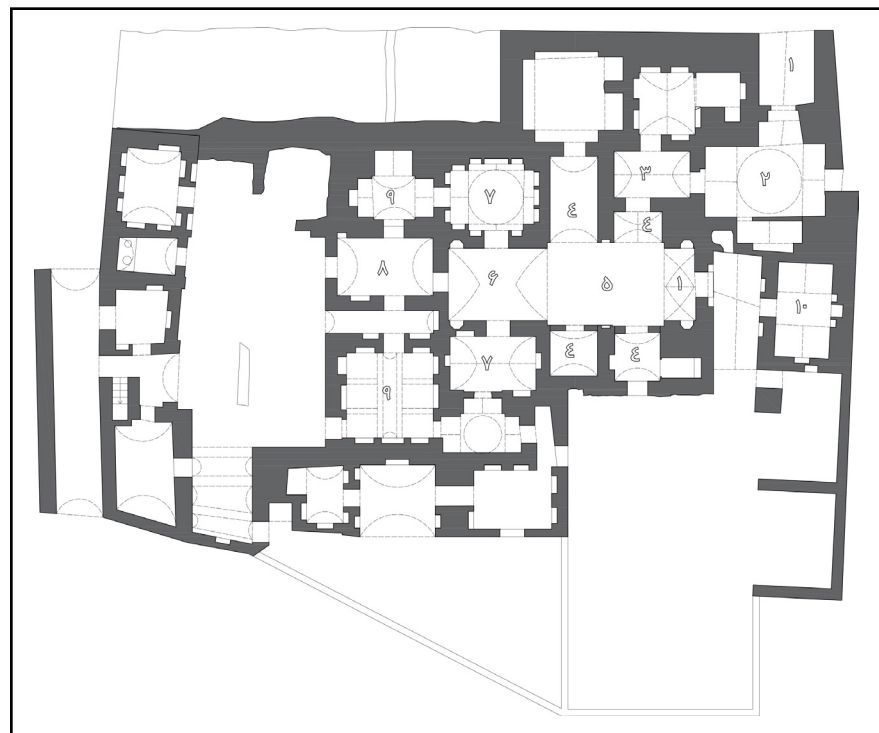
Fig. 1. Plan of ghazi Jala ad din's house in Haftador village; 1- entrance, 2- hashti, 3- hallway, 4- Eivan, 5- inner courtyard, 6- large eivan, 7- Rooms next to the large eivan, 8- tanabi, 9- room Next to the tanabi, 10- small eivan, 11- back room small eivan, 12- back yard (Archive of the Yazd Cultural Heritage Office).
