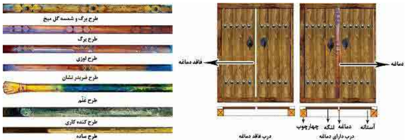
Fig. 9: Examining the types of masouleh door noses (Authors, 2023).
